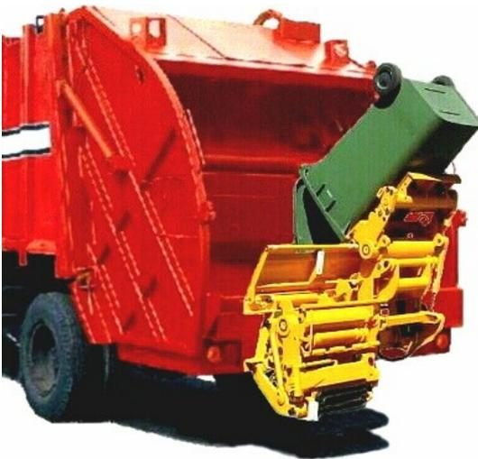
The two sides of the lifter are independently controlled when handling two-wheeled bins. On opening the trunnion arms to handle the larger four-wheeled bins, the two lifter sections are mechanically locked.
