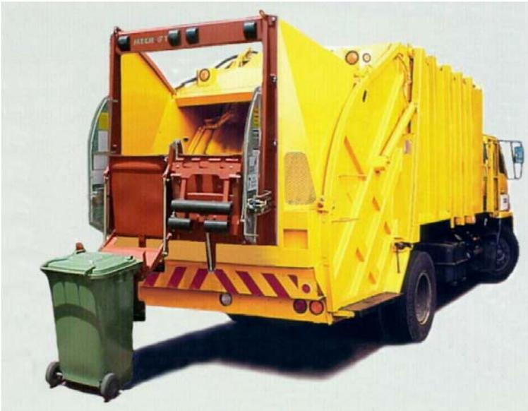
The new generation of two-wheeled plastic bins will only realize their full potential when handled by a bin lifter, which can empty over 1200 bins per 8-hour shift. The **ML220** easily does this.
